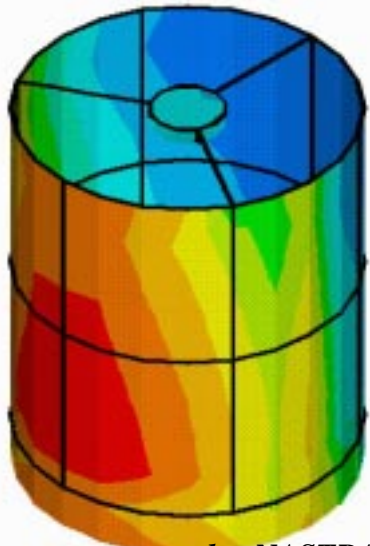
Figure 7: Temperatures mapped to NASTRAN structural model
