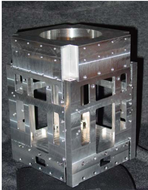
Figure 4-4: BSat EDU Structure
