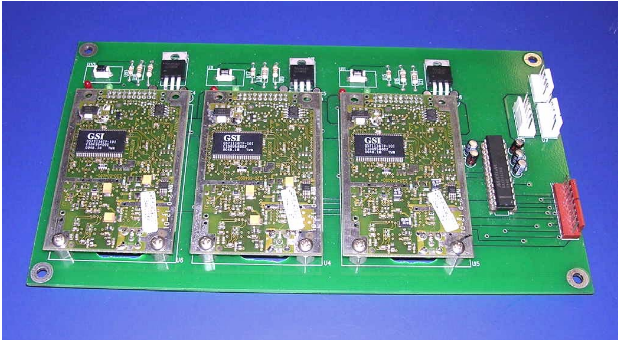
Flight prototype x3 GPS receiver and integration board.
