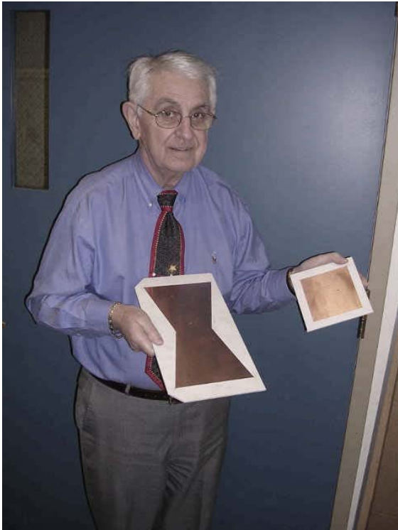
Professor Robert Labonte' holding two experimental, high performance, wide band patch antennas (140MHz left, 432MHz right).
